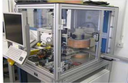
**Fig. 3.** Set-up for automated testing and training of MSM actuator elements (© ETO MAGNETIC).
